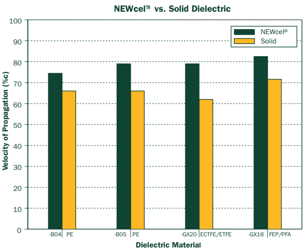
A comparison of the propagation velocity of a signal through NEWcel® and equivalent solid dielectric materials.
